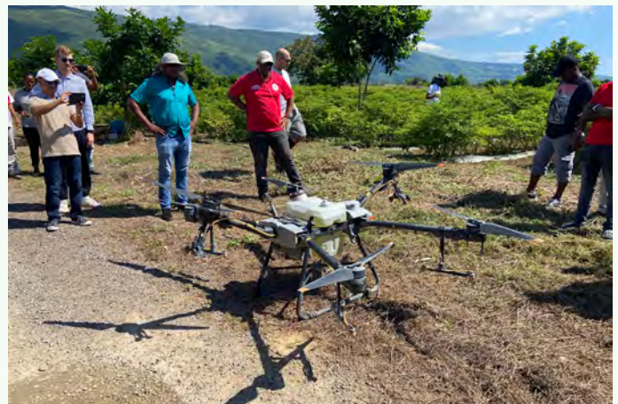
Automated drone used by GAP to spray pesticides or water
